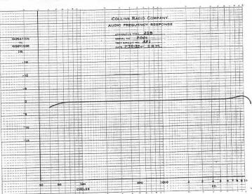
The overall audio response curve (above) was measured from transmitter input to antenna. RF modulation voltages at the various frequencies were measured on cathode-ray oscillograph in order to avoid introducing errors by the use of a linear rectifier.
