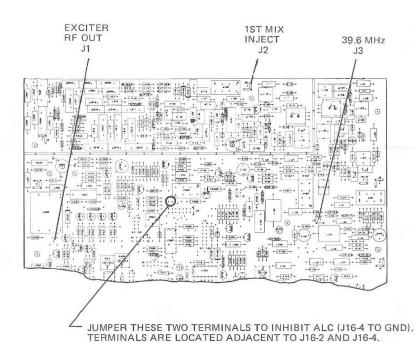
ALTHOUGH SOME COMPONENT LOCATIONS MAY DIFFER DUE TO CIRCUIT BOARD CHANGES, LOCATION OF ALC INHIBIT TERMINALS IS AS SHOWN HERE.
